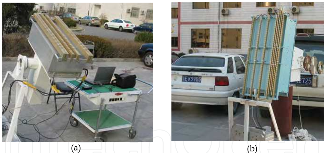
Fig. 8. One dimensional interferometric radiometers built by CSSAR
