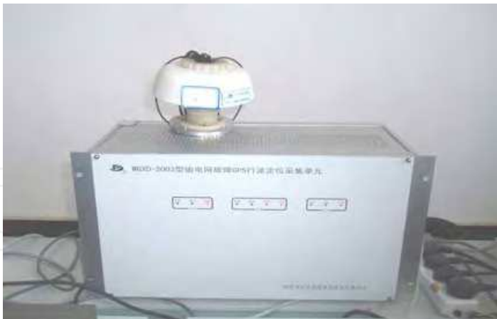
Fig. 34. Traveling wave detection device
