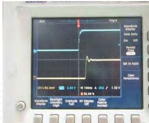
Fig. 26. Modulating pulse and video out after 100nsec delay
