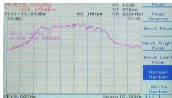
Fig. 27. The experimental results of wide band WGN in output of x-band amplifier1 on the spectrum analyser.
