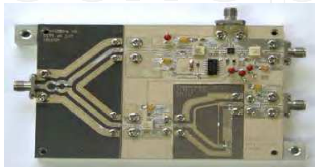
Fig. 11. Photo of 100nsec compensated delay block without cable
