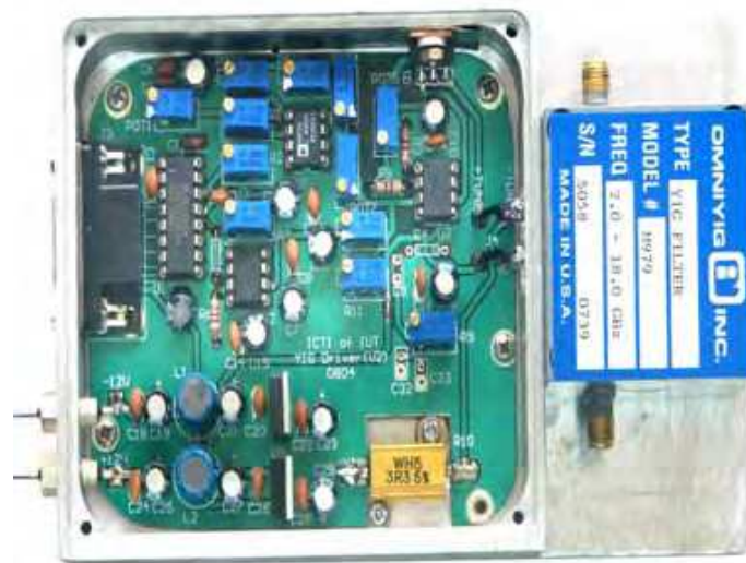
Fig. 19. Photograph of YIG filter and driver
