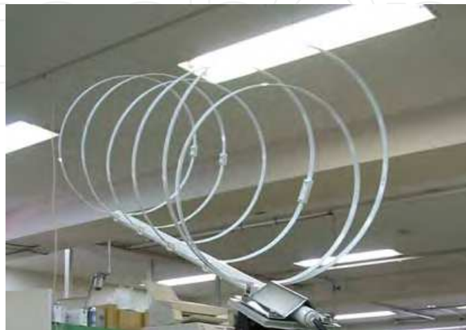
Photo 2. Right-hand Circularly Polarized Ring Loop Antenna
