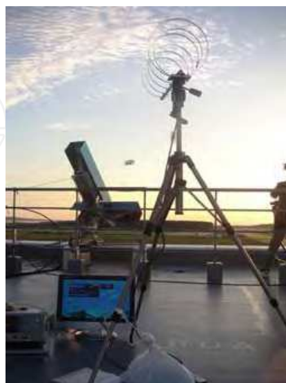
Photo 3. An antenna of the digital Right- hand Terrestrial broadcasting experiment Ring Loop with the airship in NICT
