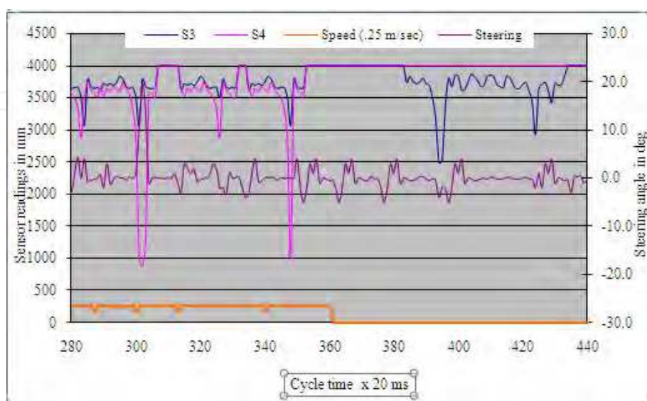
Fig. 10. Enlarged portion of Figure 9 between cycle times 280 X 20 to 440 x 20 ms plotted against obstacle distances from robot, steering angle and speed of the robot.
