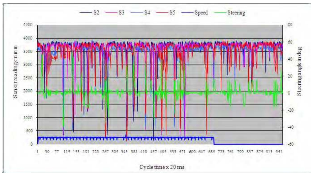
Fig. 12. Cycle time drawn against the responses of sensors S2, S3, S4, and S5 in terms of obstacle distances from robot, steering angle, and speed.
