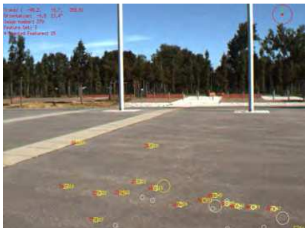
Fig. 11. A screenshot of the SSVL algorithm at work. Only close landmarks are used.
