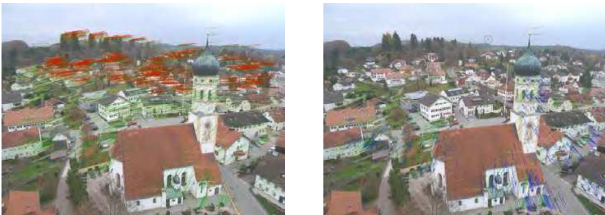
Fig. 20. Motion estimation based on SURF features.
