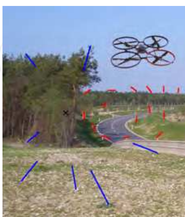
Fig. 1. The Z_{\infty} algorithm estimates the rotation (red landmarks) and the translation up to scale (blue landmarks) based on a monocular camera in an efficient way. Therefore, it fits well for resource-limited systems like e.g. flying mobile robots.
