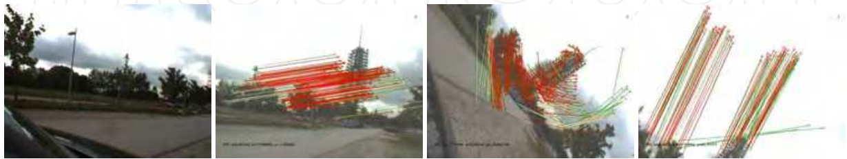
Fig. 16. These four images were used for camera to IMU calibration.
