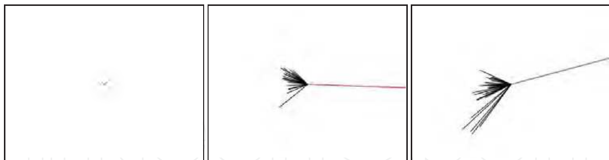
(b) These are the corresponding obstacle maps to the images above - the red line is the suggested swerve direction for obstacle avoidance.
