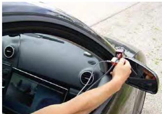
Fig. 15. The Xsens IMU is mounted on a Guppy camera. The data sets were acquired by holding the camera-IMU system out of a car.
