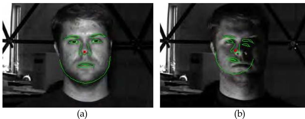
Fig. 1. Face alignment using standard AAM under good and extreme illumination. (a) Normal illumination, (b) Extreme illumination.
