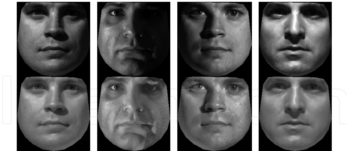
Fig. 2. Illumination normalization using histogram fitting: On the top the input images are given, and on the bottom the normalized images are shown.
