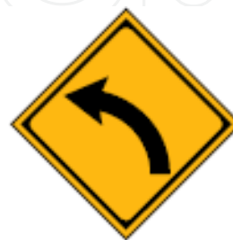
(b) An example of caution signs (existence of left curb ahead).
