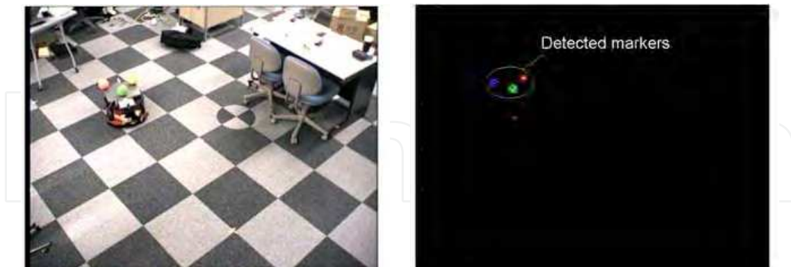
Fig. 6. Detection of color markers on a mobile robot using a camera
