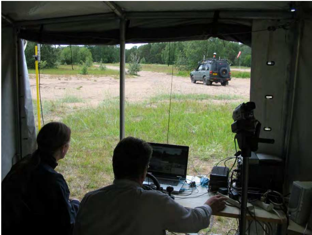
Fig. 8. Setup for the teleoperation tests. Observing researcher sitting on the left and test operator using the remote control devices on the right. The UGV starting the mission can be seen in the background.
