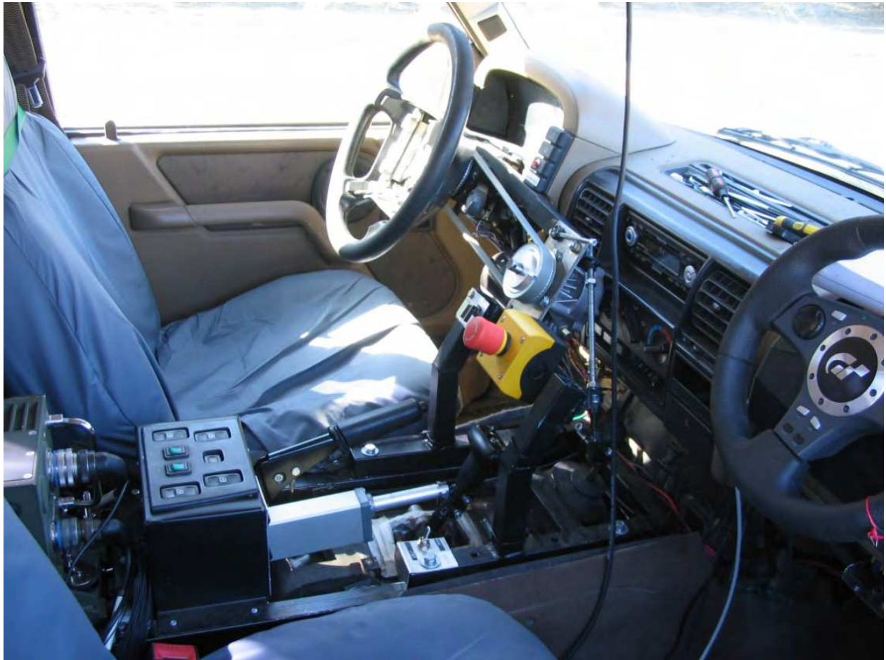
Fig. 3. Steering wheel is instrumented with brushed DC-motor and belt-pulley arrangement. Gear lever is instrumented with a spindle motor. Instrumentation was tested and the controllers were tuned by using the steering wheel shown on the right.
