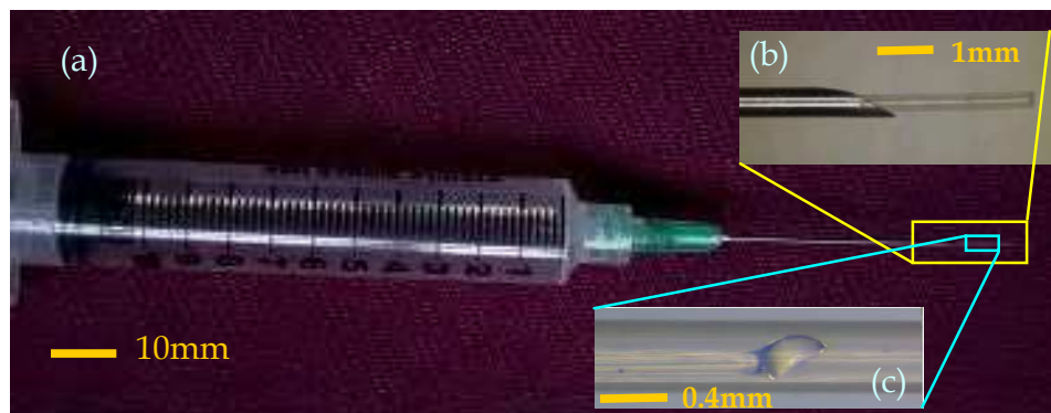
Fig. 13. OCT side-view needle probe showing the tubing and angle-polished ball lens. (a) needle probe. (b) retracted needle tip with protective tubing. (c) protective tubing and exposing the lens.
