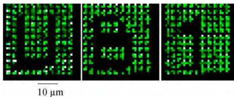
Fig. 4. THG readout of the three layers containing the bit patterns U, B, and 1, recorded in the bulk of the glass (bit spacing, 3 nm; layer spacing, 10 nm). Laser writing parameters: I = 6 \text{ TW}\cdot\text{cm}^{-2} , N = 10^6 . The three THG images present high signal-to-noise ratio and no cross talk.
