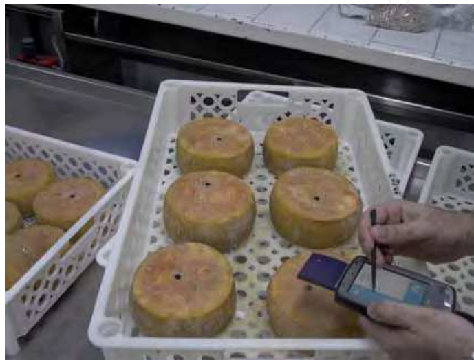
Fig. 11. Data update in cheeses with attached RFID tags
