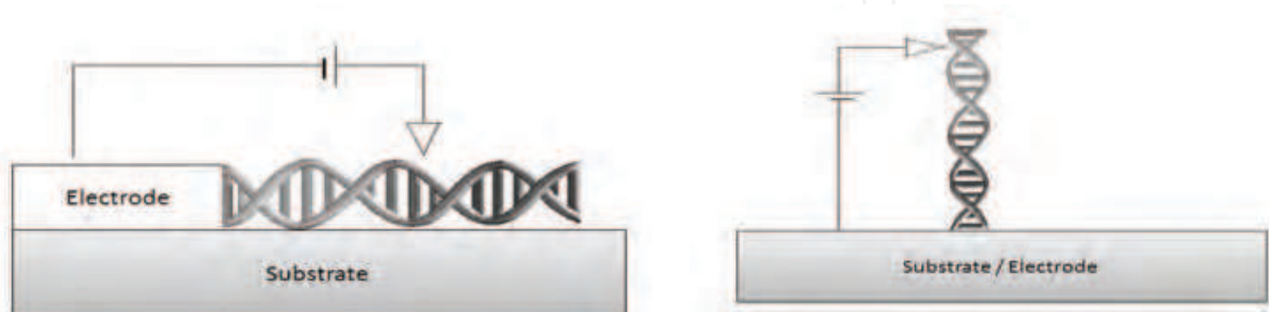
Fig. 19. The substrate is insulating in the left case; the figures depict the measurement of I - V characteristics of DNA using SPM techniques (Felice et al., 2007)
