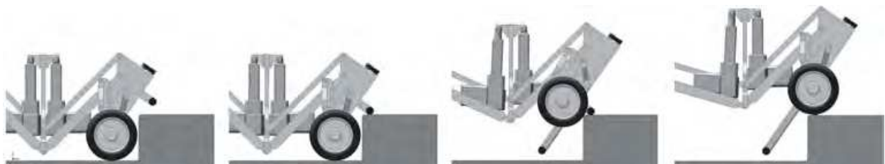
Fig. 4. Climbing sequence for the rear axle
