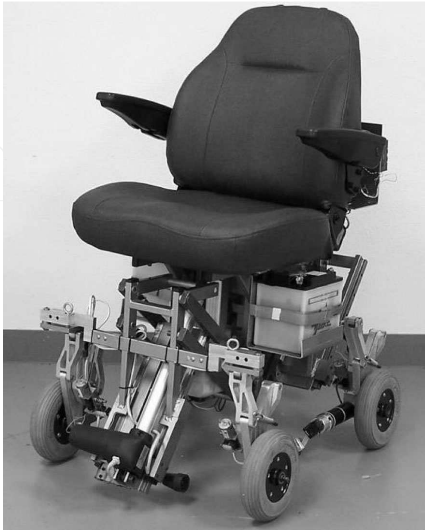
Fig. 2. The staircase climbing mechanism proposed
