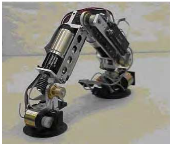
Fig. 3. RAMR1 biped climbing robot (Tummala et al. (2002))
