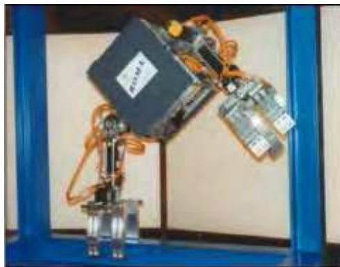
Fig. 8. ROMA1 robot climbing a beam-based structure (Balaguer et al. (2005))
