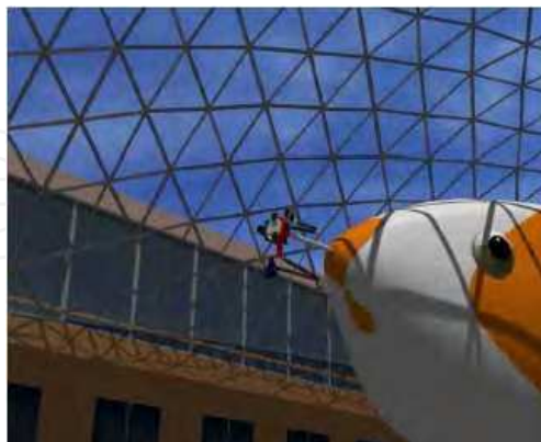
Fig. 19. Balloon-based robot consisting of a walking mechanism and a cleaning tool (Elkmann et al. (2002))
