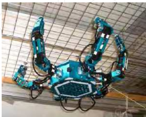
Fig. 11. ASTERISK robot hanging from a grid-like structure (Inoue et al. (2006))
