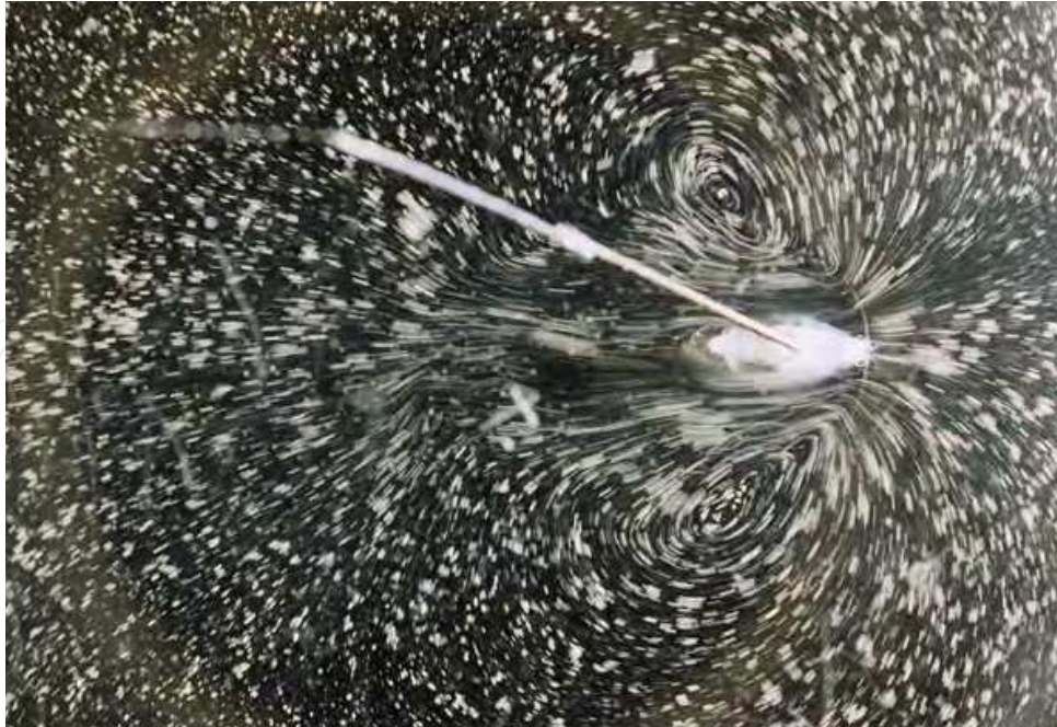
Fig. 20. Flow visualization around a tethered opossum shrimp in dorsal view
