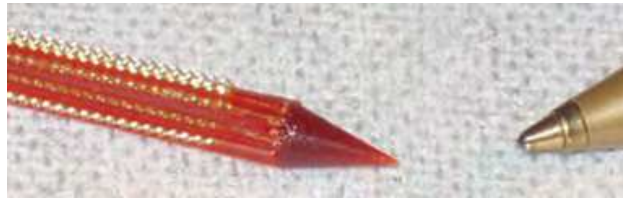
Fig. 4. Picture of the brain probe prototype (left) and pen as size reference (right) Frasson, Parittotokkaporn, Davies & Rodriguez y Baena (2008).
