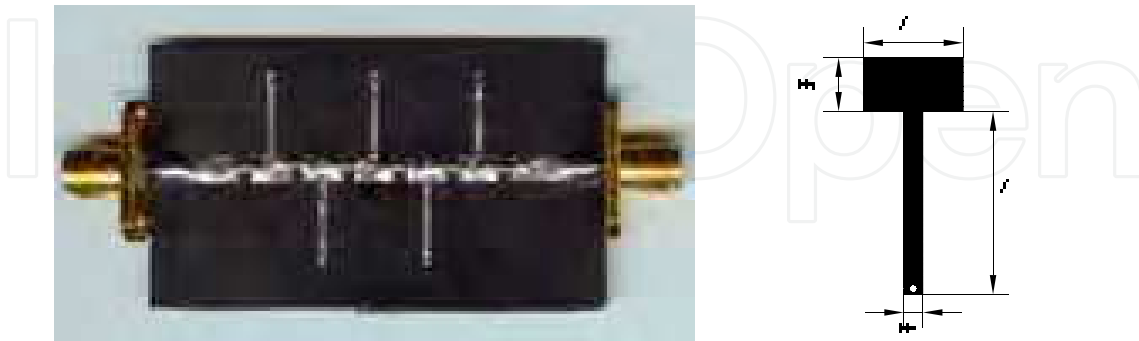
Fig. 7. A composite right/left-handed transmission line with lumped capacitors and the microstrip structure
