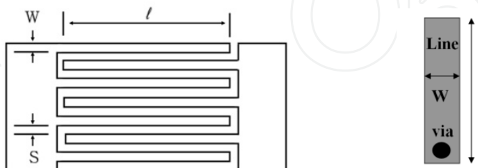
Fig. 2-3. Microstrip interdigital coupled lines and grounded stub
