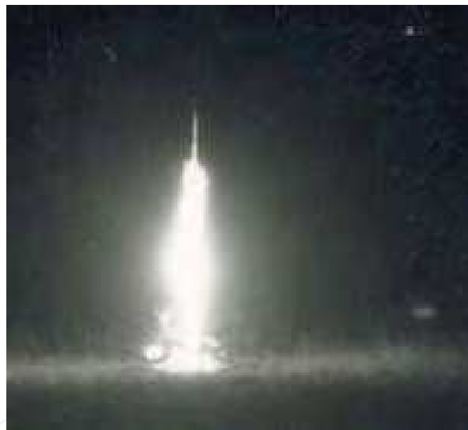
Fig. 17. Plasma dielectric antenna based on shaped charge with cylindrical liner.
