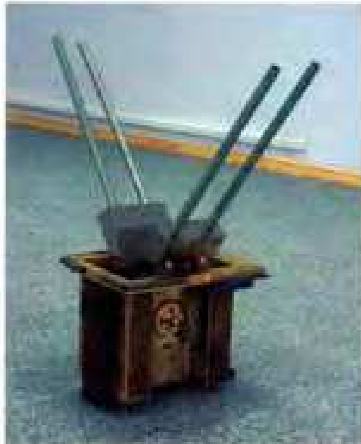
Fig. 2. Plasma dielectric antenna with four jet [8].
