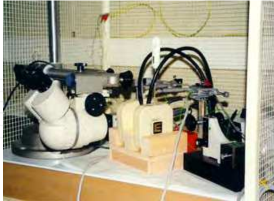
Fig. 6. Experimental set-up for application of ELF-MF. The neuron sample is placed between a pair of Helmholtz coils.
