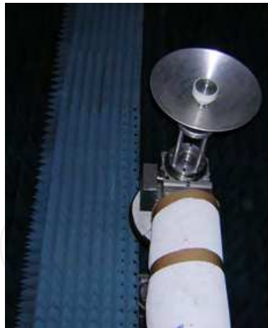
Fig. 6. Ku-band reflector employed for the validation measurements
