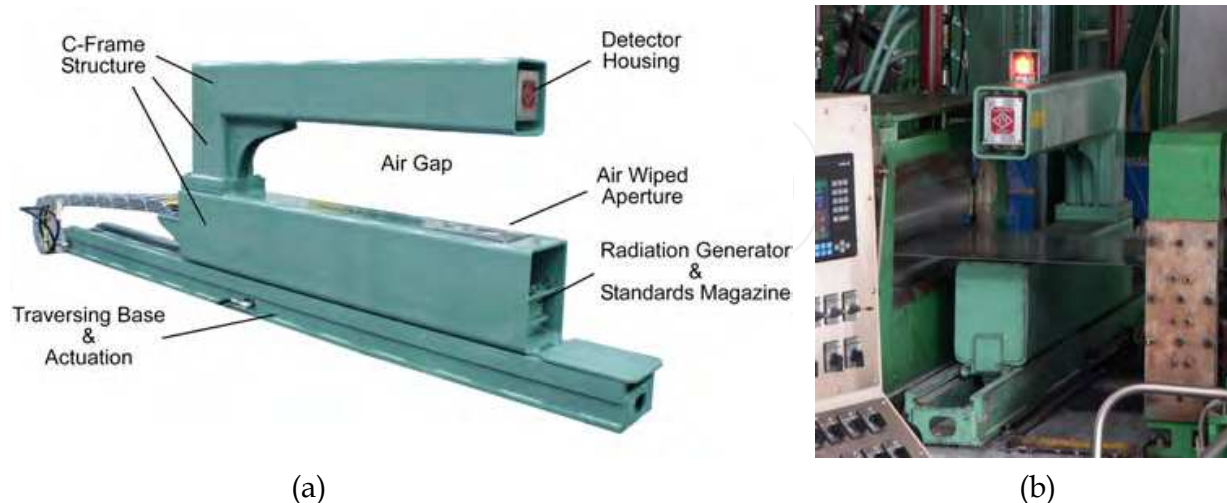
Fig. 8.1 - Photo diagrams showing various C-Frame arrangements: a) Primary components, b) C-Frame in flat strip application.
