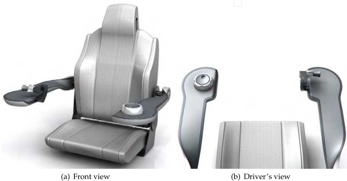
Fig. 3. Intuitive operational concept for hydraulic excavators
