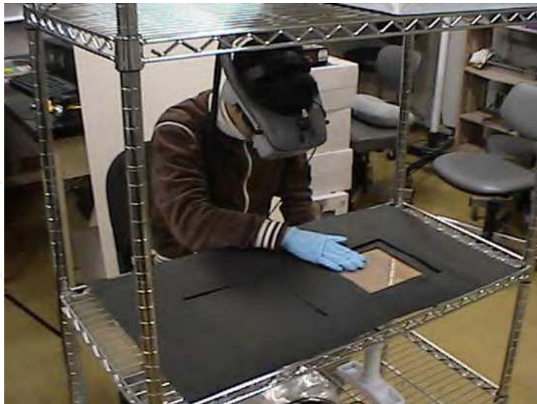
Fig. 5. An Experimental Scene of Evaluation. We use a glove that deadens the haptic sensation to maintain balance of haptic and visual stimuli.
