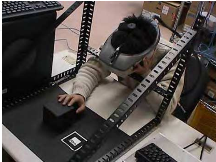
Fig. 9. Experimental of Subjective Evaluation of Sharpness. The subject maintains his viewpoint while putting his jaw at a predefined position to preserve geometric and photometric consistency between the real and virtual information.
