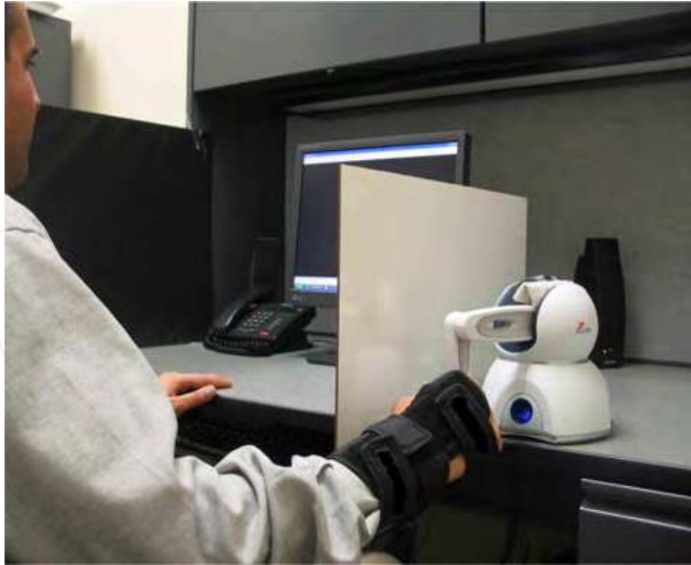
Fig. 5. The subject grasps the end-effector of the PHANTOM TM Omni and rotate his hand about his elbow.
