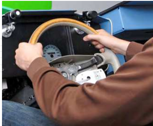
Fig. 3. A close-up of a subject holding the steering wheel, which could be perturbed or which could provide haptic guidance. The human reaction torque T_c and the resulting angular rotations X_c were measured.
