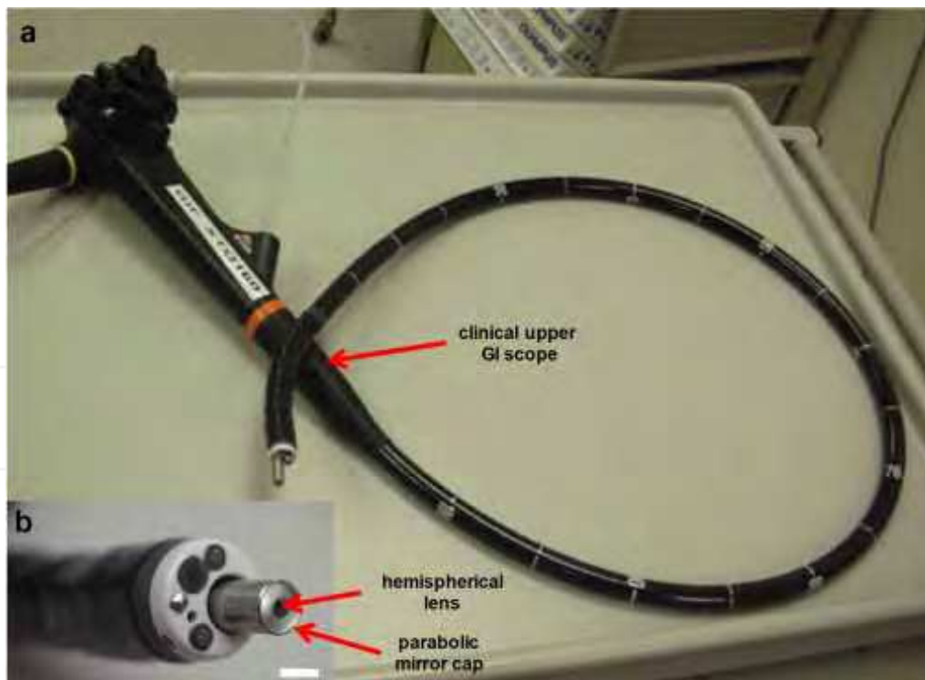
Fig. 24. Endoscope-compatible dual axes confocal microscope. a) Microscope passes through the instrument channel of an Olympus XTQ 160 therapeutic upper endoscope that has a 6 mm diameter instrument channel. b) Distal end of endoscope shows the protruding dual axes microendoscope.
