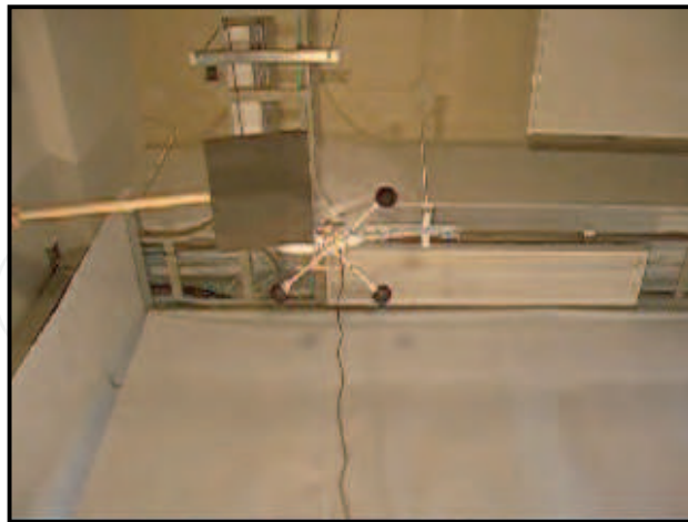
Fig. 8. A snapshot of helicopter flight under an occlusion. This was captured by a camera placed next to camera 2. Ball 3 was not captured correctly at this moment.
