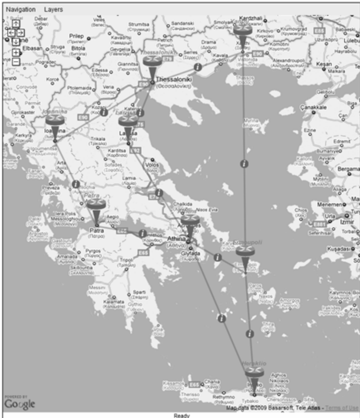
Fig. 1. GRNET's Layer 3 Country Network Topology
