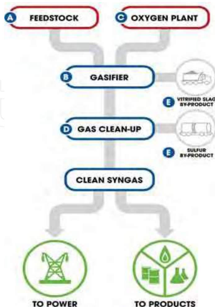
Fig. 7. A schematic diagram of gasification process
