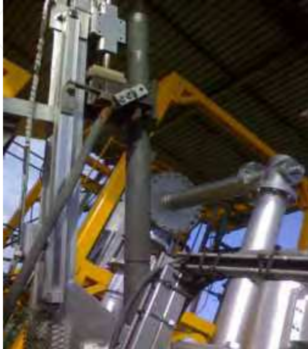
Photo 9. Movement Mechanism of the graphite electrode
