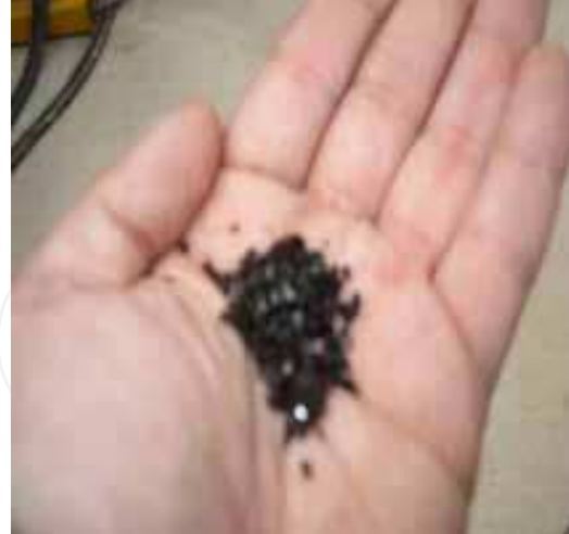
Photo 15. Water cooled slag in the form of granules
