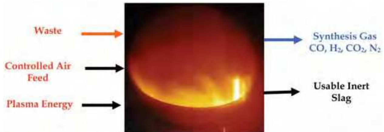
Fig. 10. A schematic diagram of plasma process
