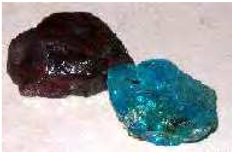
Fig. 10. Vitrified contaminants aspect after PPV reaction ( http://paginas.fe.up.pt/~jotace/gtresiduos/plasmapirolise.htm ).
