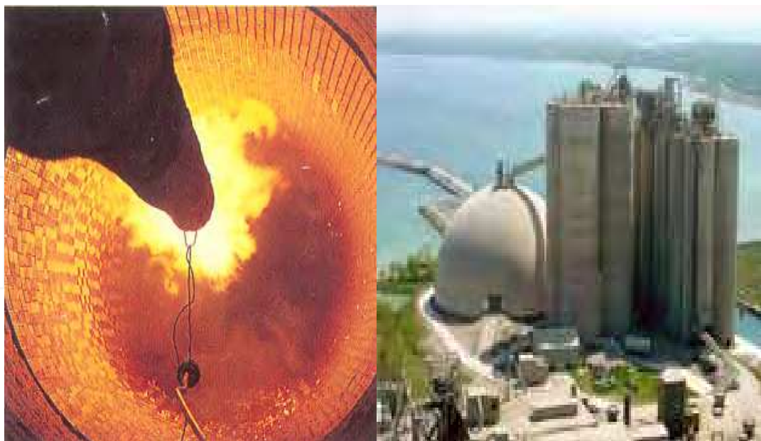
Fig. 6. Picture of inside (left) and outside (right) of a co-incineration unit in cement furnace used to burn dangerous industrial solid wastes (Puna, 2002).
