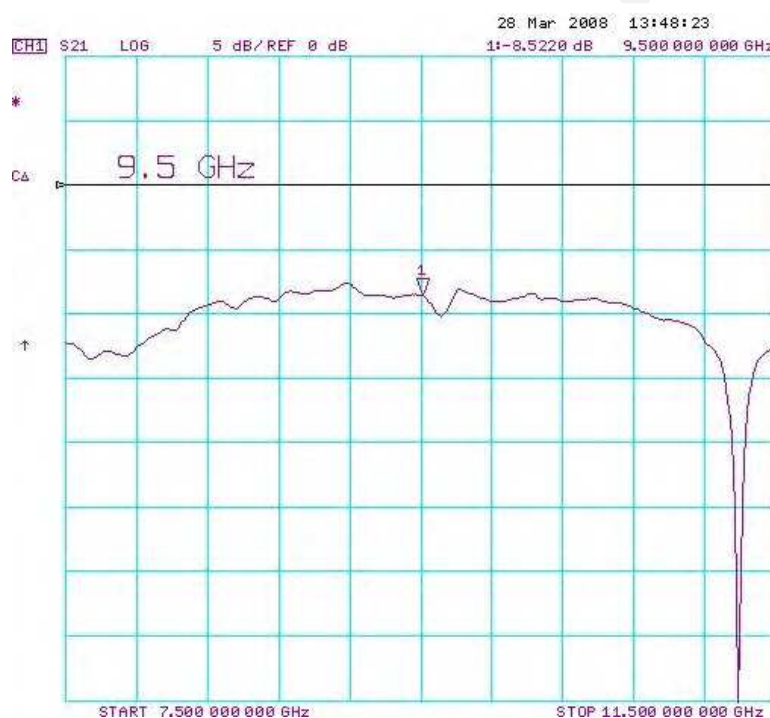
Fig. 15. Example of measurement results – transmission characteristics from centre coax input to one of coax output port
