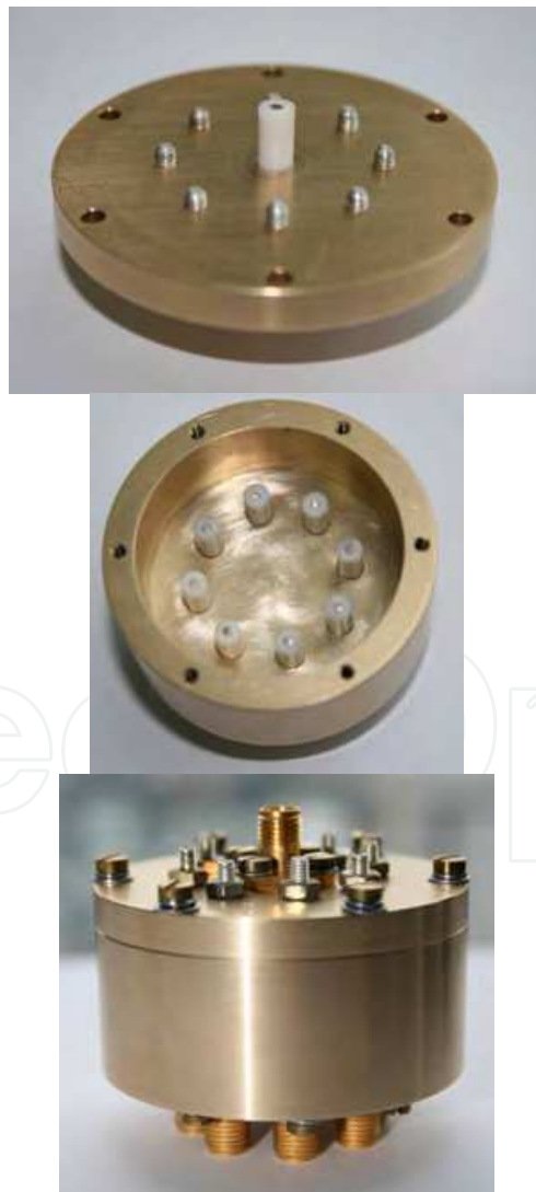
Fig. 14. Manufactured model structure of nine-port power splitter/combiner
