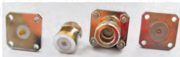
Fig. 17. Measurement kit: a panel N connector, a measurement probe and open and short calibration standards
