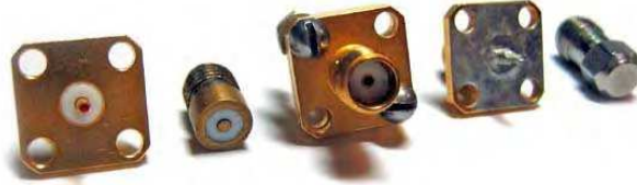
Fig. 18. Measurement kit: a panel SMA connector, a measurement probe, open, short and matched ( 50\ \Omega ) load calibration standards
