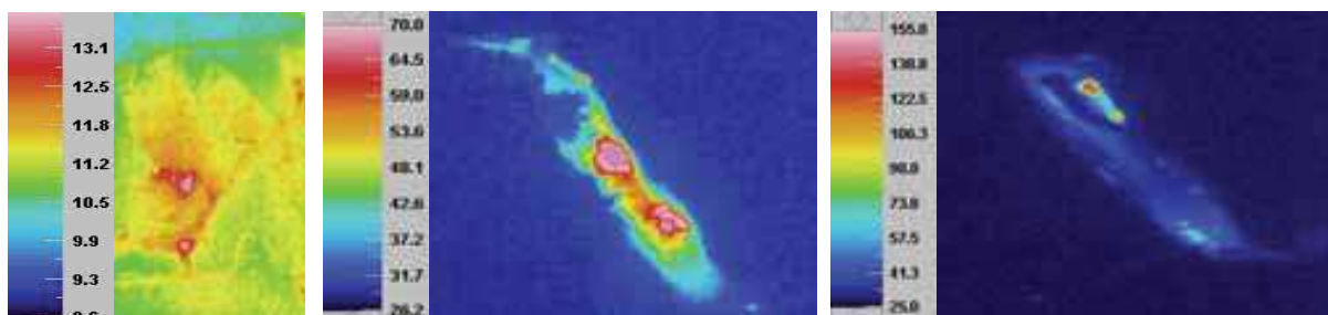
a) uni-axially loaded granite b) compressively sheared gabbro-1 c) compressively sheared gabbro-2
