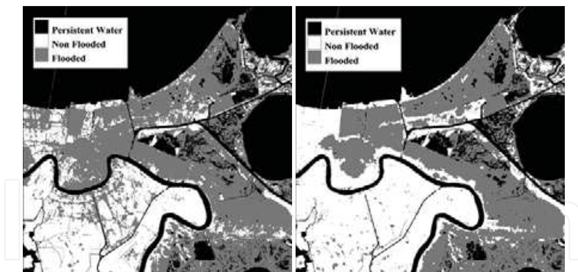
Fig. 15. New Orleans (Louisiana). Global damages mapping using the ST-MNF technique. (left) Derived from SPOT-4/HRVIR data; (right) Derived from Landsat-5/TM data.
