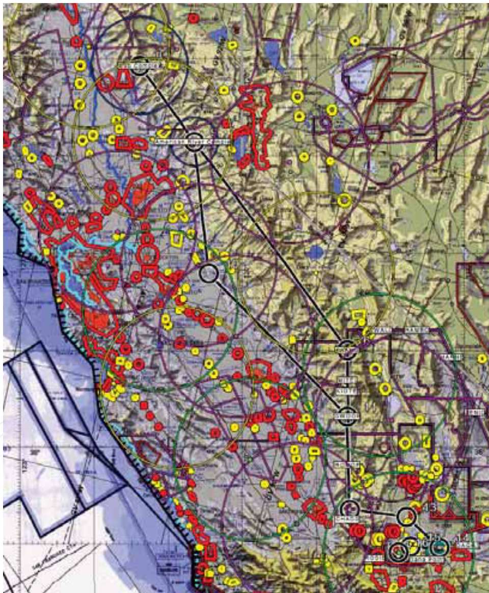
Fig. 6. Flight Plan for FAA defining Ikhana fire imaging mission route (black line), UAS turn / linger points (small black circles), tertiary landing locations along flight route (purple circles), restricted-flight / no flight zones (yellow / red polygons), and major lingering imaging locations (fire areas) (blue circles). Data displayed on a digital air navigation chart.
