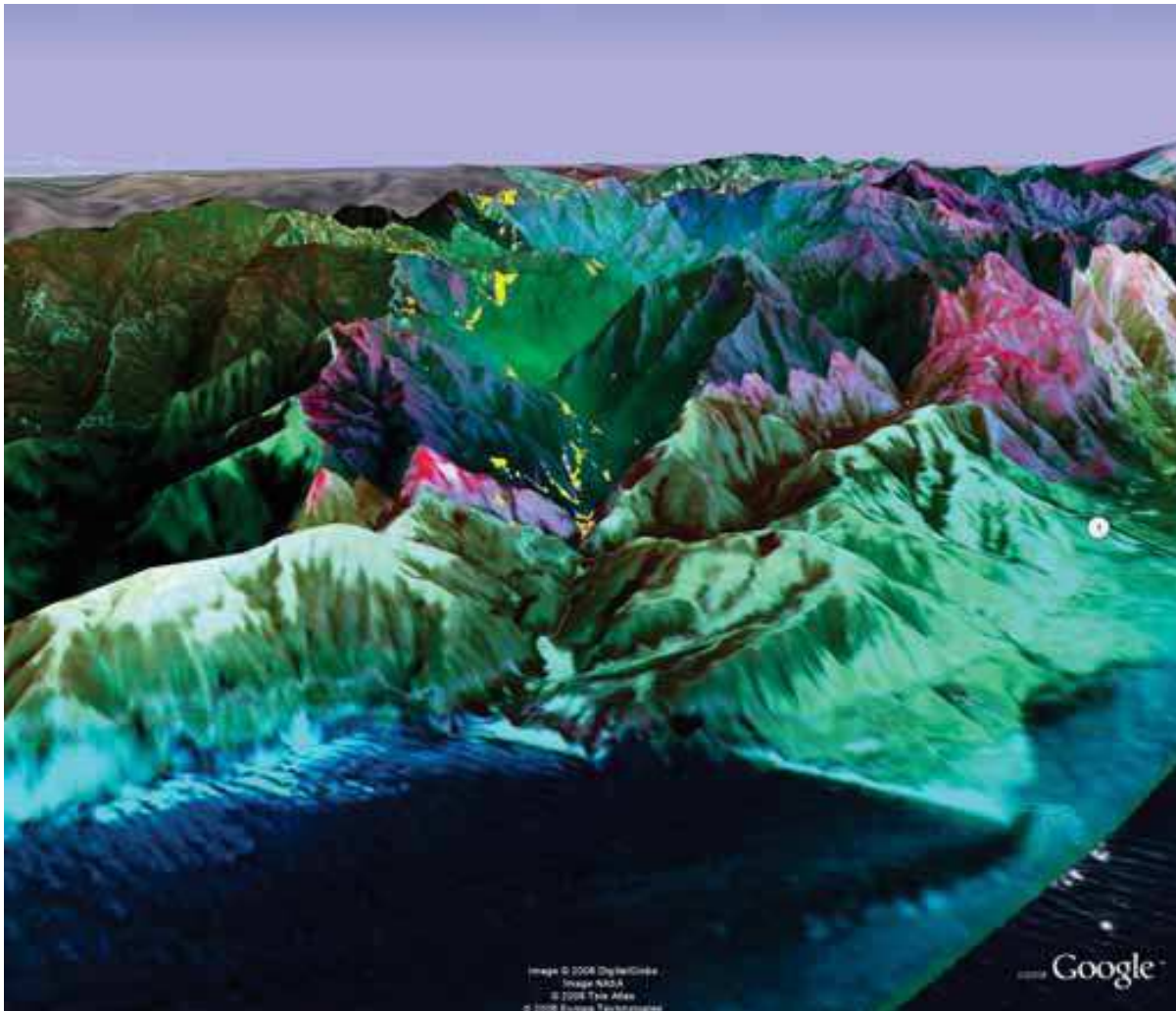
Fig. 11. Three-dimensional view of AMS-Wildfire sensor imagery collected on 8 July 2008 over Basin Fire Complex, California. This eastward looking view shows the hot-spot fire detects (yellow polygons) overlain on the three-band color composite, which is draped on the GoogleEarth background data base. Note the locations of the fire on the south-facing (sun-intense) slopes at this data collection time.
