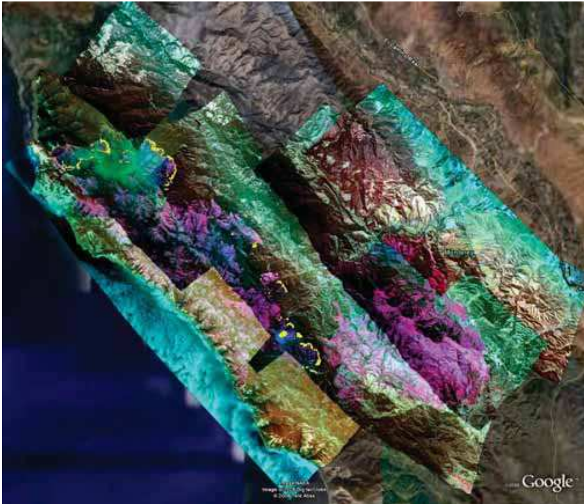
Fig. 9. AMS-Wildfire sensor near-real-time processed image “segment” mosaic for the Basin Fire Complex, Big Sur, California, collected on 8 July 2008. Data was processed and mosaiced in “real-time” from 5 flight lines of 22 segments of AMS data. The fire hot-spot detection algorithm shape-file information, shown draped in yellow, on the 3-channel composite mosaic (which is draped on the GoogleEarth W-CDE).
