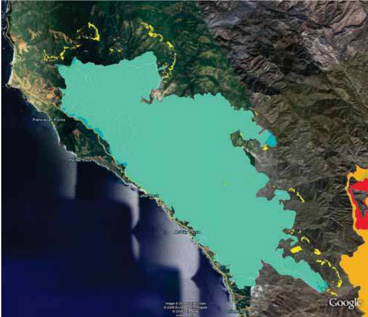
Fig. 10. AMS-Wildfire sensor data collected 8 July 2008 over Basin Fire Complex, California. The hot-spot vector file data (yellow polygons) are shown overlain with the recent fire perimeter polygon (teal). All layers draped in GoogleEarth for visualization. The yellow hot-spot fire fronts can be seen extending outside the fire perimeter.
