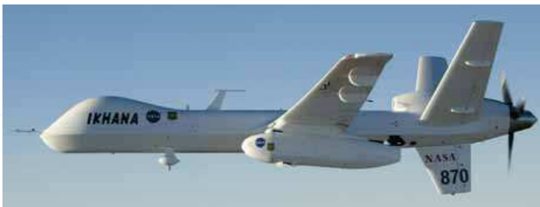
Fig. 2. The NASA Ikhana UAS with the sensor pod mounted under the left wing.
