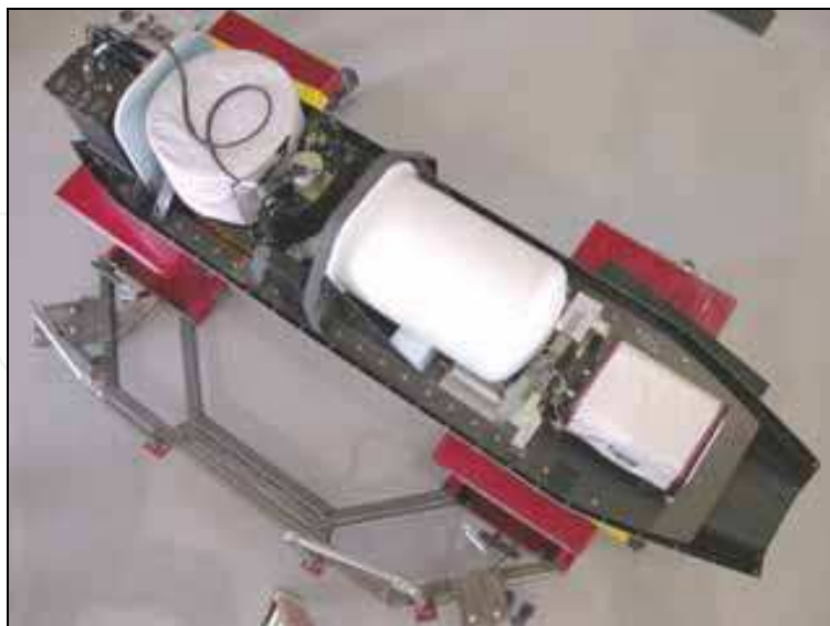
Fig. 3. The NASA AMS-Wildfire instrument arranged in the sensor payload pod tray. The scan-head is located under the cylindrical white thermal blanket at the top-left of the pod tray, while the white pressure vessel in the center contains the digitizer and electronics. Other components include the power supply and various controlling electronics.
