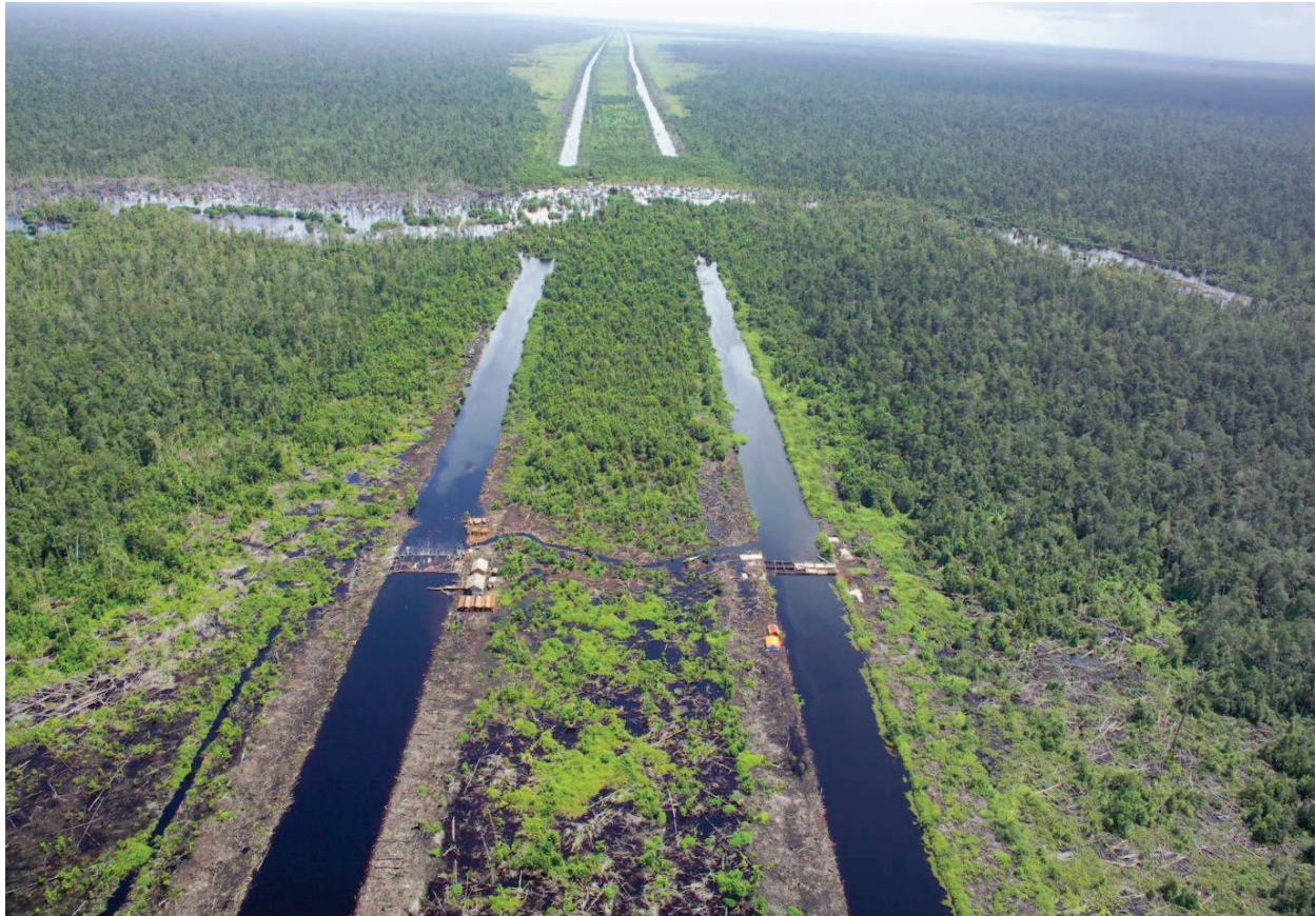
Fig. 6. Low altitude aerial photograph of the main East-West oriented double canal system passing South of Mawas. It shows the crossing of the Mentangai river, canal blocking activities and stretches of burnt forest areas along the canal, covered with small bushes and ferns. January 2005. Courtesy: Ruandha Agung Sugardiman, Indonesian Ministry of Forestry.
