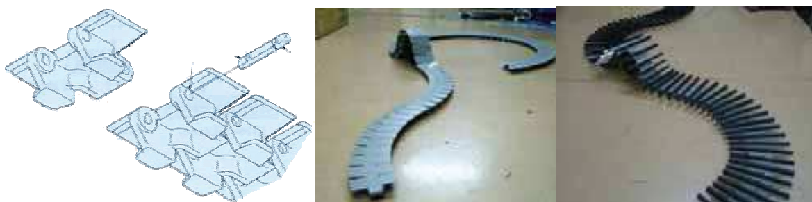
Fig. 6. Flexible belt: Configuration of belt segments (the left), Flexible belt (the middle) and belt with grousers (the right)
