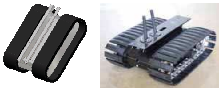
Fig. 4. Differential tracks, the right figure is 'Frigo-D' developed by National Research Institute of Fire and Disaster
