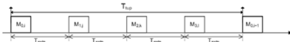
Fig. 16. TDMA round indicating the slots allocated to each robot.
