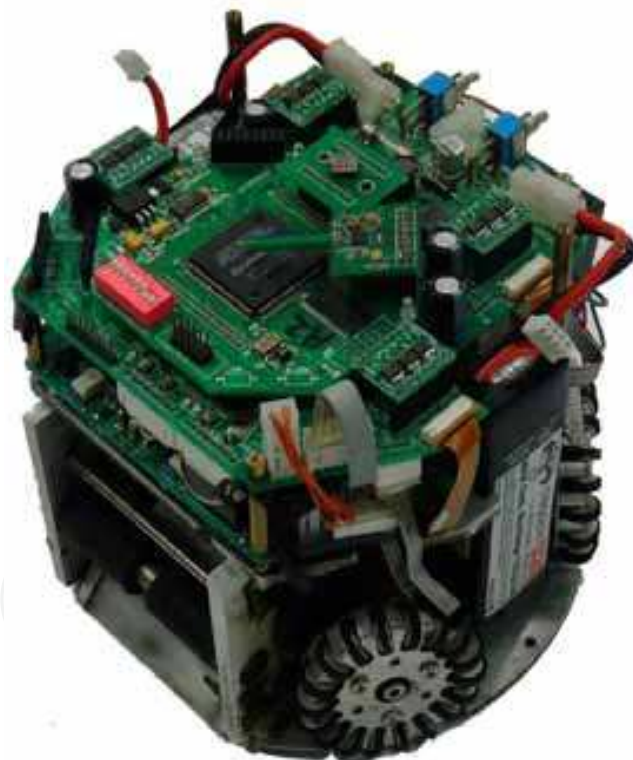
Fig. 4. The Soccer Robot with Electronic Control system.
