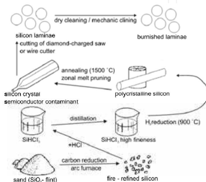
Fig. 20. Silicon production cycle (Limbra M. and Poulek V. 2006).
