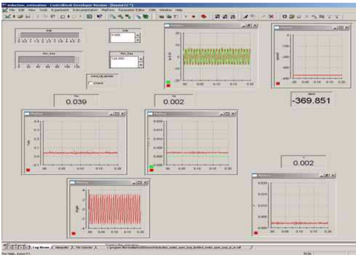
Fig 24. Real-time simulation results using dSpace Control Desk
