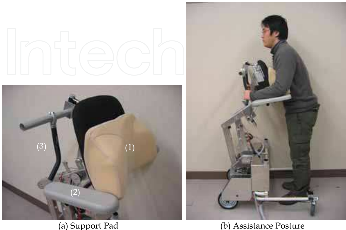
Fig. 3. Our proposed support pad. (1) is the pad with a low repulsion cushion, (2) is the arm holder and (3) is a handle. Its diameter is 0.24[m] which is easy to grip for the elderly. Our support pad has force sensors in its body.
