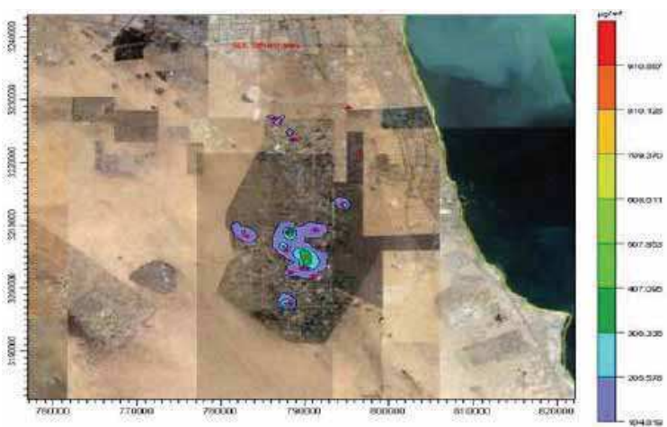
Fig. 3b Isopleths plot for the maximum daily average ground level concentrations of non-methane hydrocarbons in \mu\text{g}/\text{m}^3
