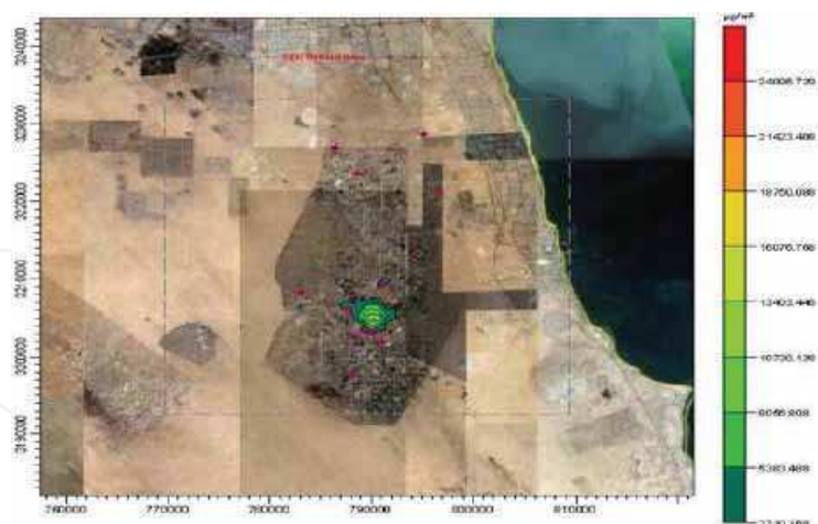
Fig. 3a Isopleths plot for the maximum hourly average ground level concentrations of non-methane hydrocarbons in \mu\text{g}/\text{m}^3
