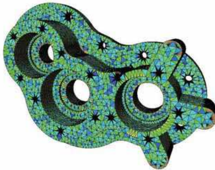
Fig. 10. Pump carter [17]. Colormap according to quality of triangles.
