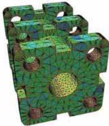
Fig. 15. Support of an axle. Colormap according to size of the triangles
