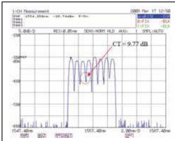
Fig. 16. The crosstalk measurement for 8-channels AWG-based OCDMA encoder
