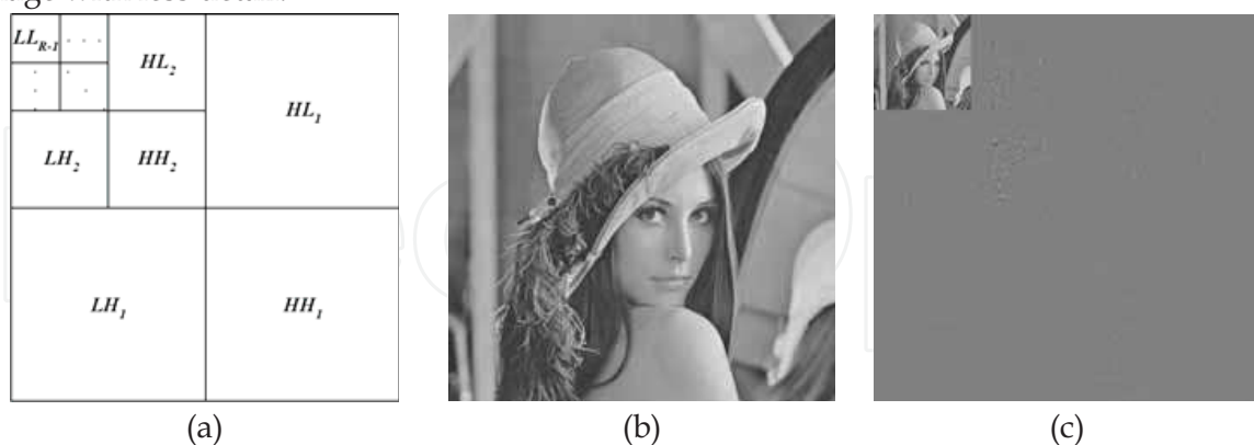
Fig. 1. DWT; a) Sub-band structure, b) Lena, c) Lena at level 2 DWT decomposition.
