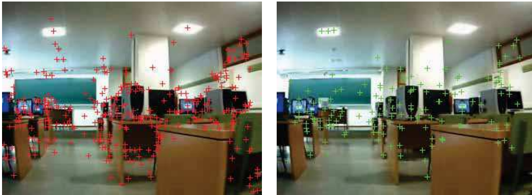
Fig. 5. SIFT (left) and SURF (right) keypoints computed on the same frame.
